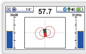
**Sonde location** - When directly over the sonde the sonde icon appears and depth is shown in upper left
